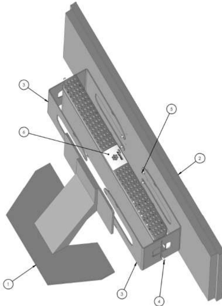
3. Attach the unit to the bracket using the four small screws (8-32 x 3/8) provided with the bracket.
