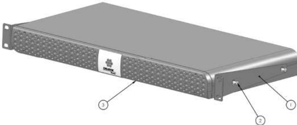
2. Attach the rack mounting brackets to the rack rails using the four large screws (10-32 x 3/4) provided in the install kit.
