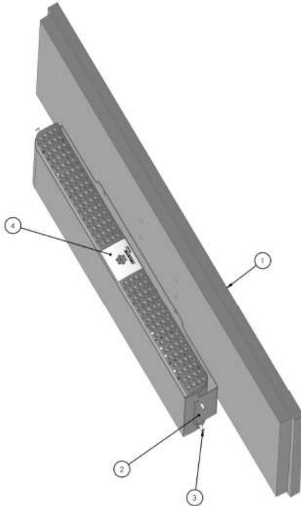
2. Attach the bracket to the monitor using the appropriate hardware.
