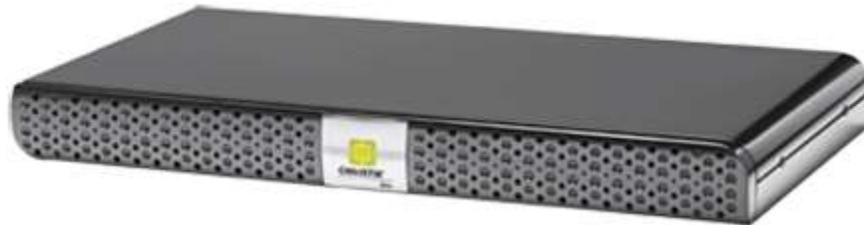
When the LED indicator on the front of the unit is solid green, the unit is ready. The LED flashes when the unit is powering on.
