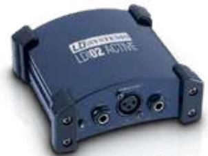
Active DI box in sturdy metallic blue/silver aluminium and steel housing with corner protectors, internal 9 V battery (indicator blinks during operation) which is automatically switched off when phantom power is used (indicator is on continuously). Extremely low battery consumption, 9 V battery not included.
